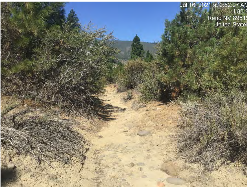
Photograph 58: Wash with N value of 0.035 contains cobbles, sand, silt, and pebbles. Photo facing west. Image 4398 Date: July 16, 2021
